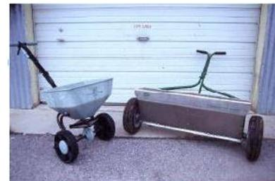
Fig. 3. Rotary (left) and drop (right) fertilizer spreaders.
