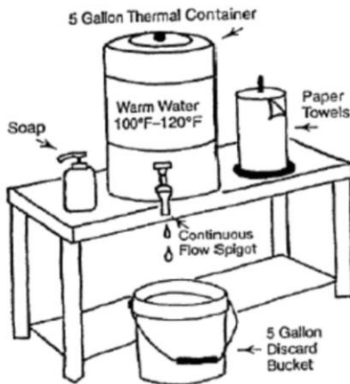
Proper Hand Wash Station
